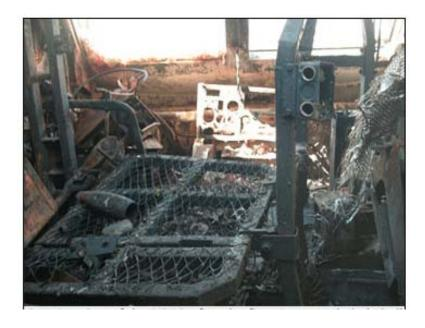
Interior view of the MRAP after the fire. An unexploded shell body from a M768 cartridge can be seen at the lower left.
