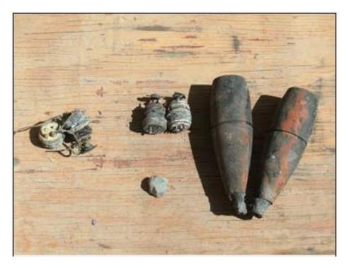
Shell bodies and separated M783 fuzes from M768 cartridges recovered from the vehicle after the fire.
